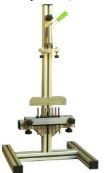
Thanks to the smart design of the EH20 quick connection device, it may be used for the connection of practically all types of electricity meters with currents up to 100A.
