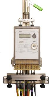
Spring contact pins of the EH20 are used to make connection to the meter and may
