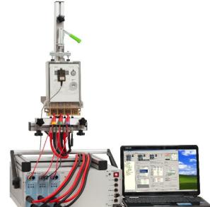
The Calmet TB10 Test Bench employs modern precision power source with the internal reference (without need to use an additional external reference energy meter with additional cables).By this conception may be achieved simultaneously flexible customer orientated solution characterised by extremely compact size, light weight, high metrological properties at reasonable price.
