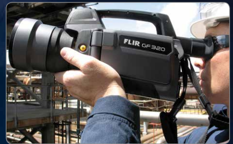
GF300/GF320 CAMERAS FIND LEAKS QUICKLY OVER WIDE AREAS
