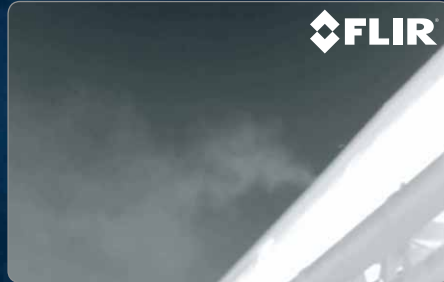
CO LEAK FROM A BLAST FURNACE
