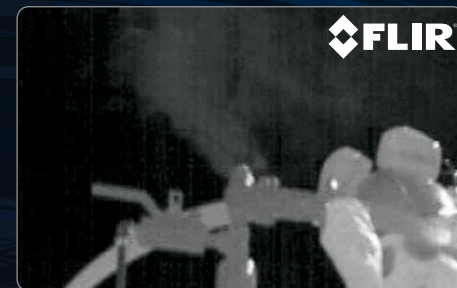
OPTICAL GAS IMAGES OF \text{SF}_6 LEAKS
