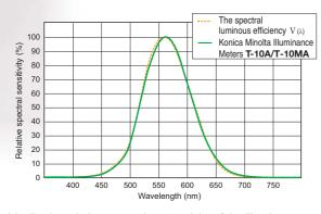
Ideally, the relative spectral responsivity of the illuminance meter should match V ( $\lambda$ ) of the human eye for photopic vision. As shown in the graph above, the relative spectral responsivity of Konica Minolta Illuminance Meters T-10A/10MA is within 6% (f1') of the CIE spectral luminous efficiency V ( $\lambda$ ).
