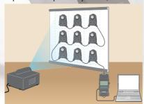
Illuminant Meter T-10A T-10A Receptor head Adapter units for Main Body T-A20
