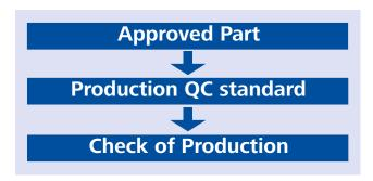
Instead of working with absolute gloss numbers, supplier production QC needs to be based on the signed-off part where only the differences are checked with the glossmeter. This procedure eliminates the reproducibility error as gloss is measured relatively on the same type of material and same surface.
