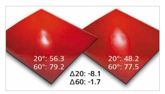
The different gloss of these two samples is more clearly shown in the  $20^{\circ}$  readings.
